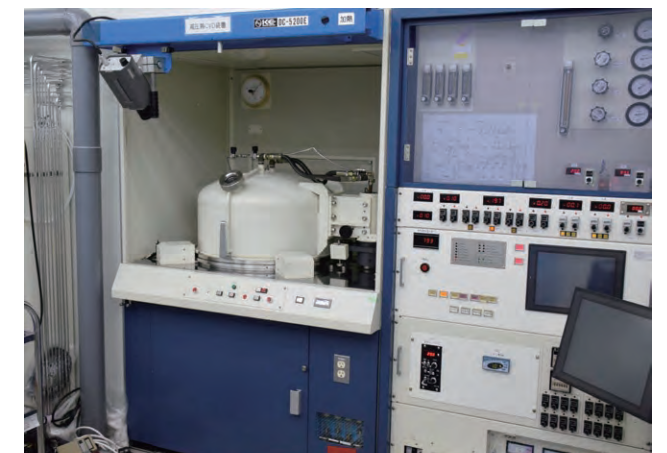
熱CVDによる低応力厚膜doped poly-Si Thermal CVD for low-stress, thick-film doped poly-Si
