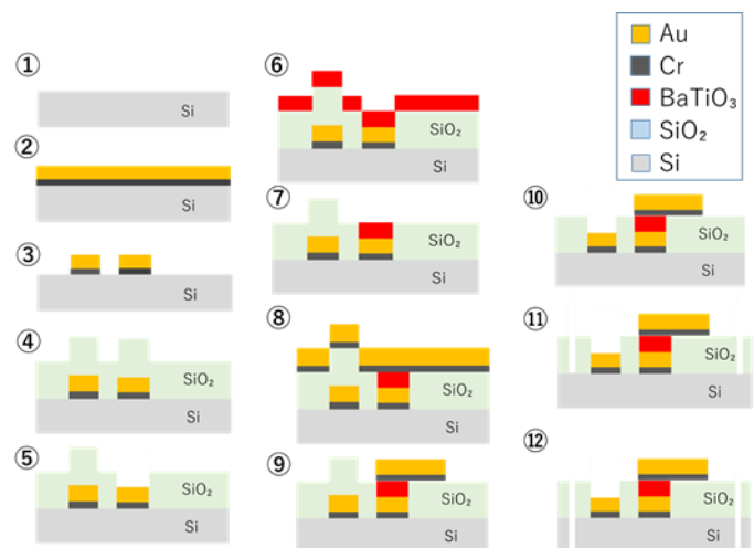
Fig.1 Schematic diagram of device fabrication
