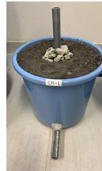
Fig. 1 Small experimental device that imitates the final disposal site
