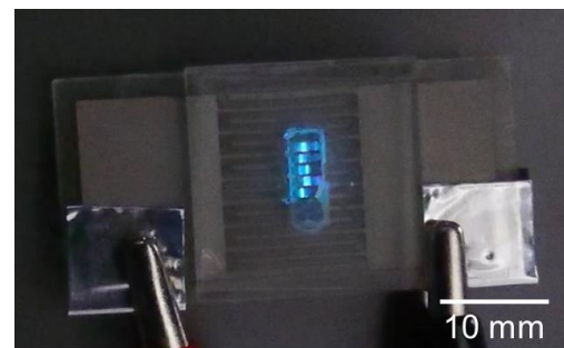
Fig. 2 Result of luminescence evaluation (applied voltage: 3 kV)
