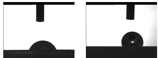
Fig. 1 Mold Release Agent Coating Results (Left) Uncoated (Right) Coated
