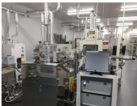
Fig. 1 Photograph of the ALD system (Picosun SUNALE R-150)
