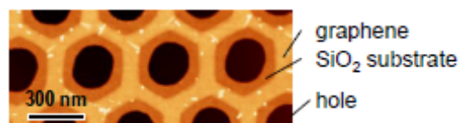
Fig. 1: Atomic force microscope image of a network of zigzag graphene nanoribbon (about 80 nm wide).
