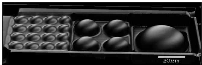
Fig. 1 Assorted size spherical lenses fabricated from a single pattern data file
