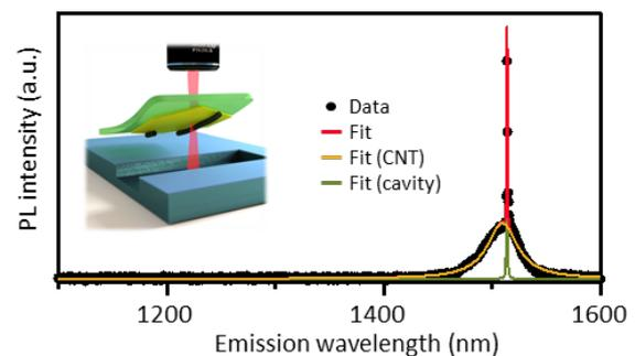
Fig. 1 Photoluminescence spectrum of nanotube emission coupled with the fundamental mode of a microcavity. Inset: Schematic showing a part of nanotube transfer process.
