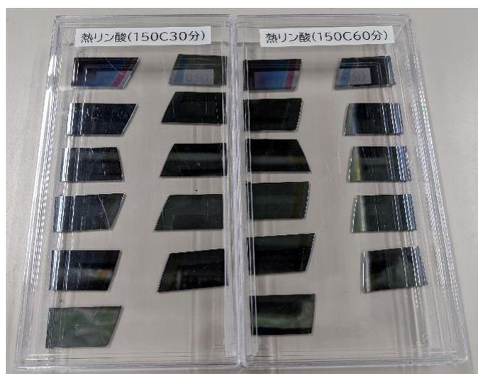
Fig. 1 Si wafer chip with SOG coating.
