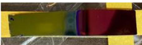
Fig.1 Pictures of Si substrates after wet etching.
