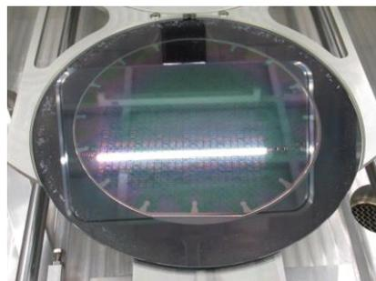
Fig. 1 TEOS-SiO<sub>2</sub> film deposited on Si.
