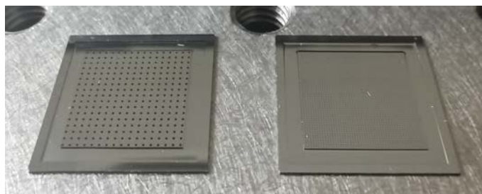
Fig. 1 Two different sizes membrane. The left is a 150 \mu\text{m} pore size membrane, the right is a 50 \mu\text{m} pore size.
