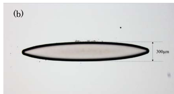
Fig.1 (a) Specimen for fatigue test ,(b)Notch image
