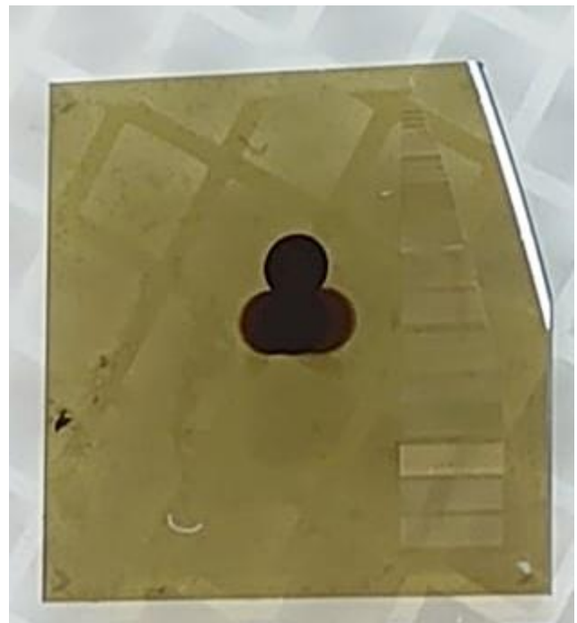
Fig. 1. 4H-SiC sample photograph after the RBS measurements by He ion and N ion irradiation.
