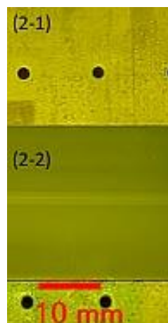
Fig. 2 (2-1) CaO 0.42 μm and (2-2) Al 0.15 μm coating on parylene film
