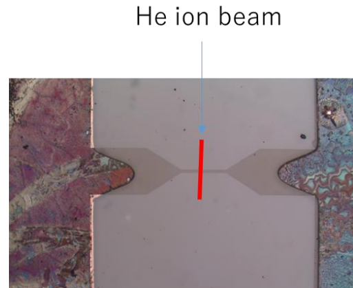
Fig. 1 Picture of 100 \mu\text{m} -long and 10 \mu\text{m} -wide MgB 2 line and the position of He ion beam irradiation.
