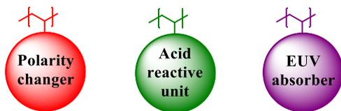
Figure 1 Schematic model of chemically amplified negative resist.
