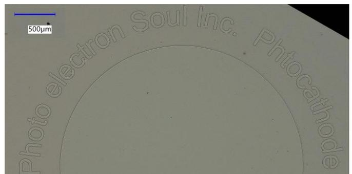
Fig. 2 Microscope image of patterned photocathode after dry etching and removing photoresist.
