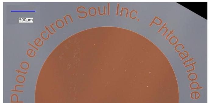
Fig. 1 Microscope image of patterned photoresist on the photocathode before dry etching.
