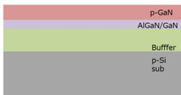
Fig. 1 Schematics cross-section of GaN on Si
