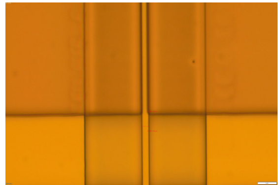
Fig. 1 Picture of the photoresist pattern on the laser diode substrate, The scan direction is parallel to the ridge waveguide.
