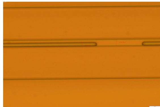
Fig. 2 Picture of the photoresist pattern on the laser diode substrate, The scan direction is perpendicular to the ridge waveguide.
