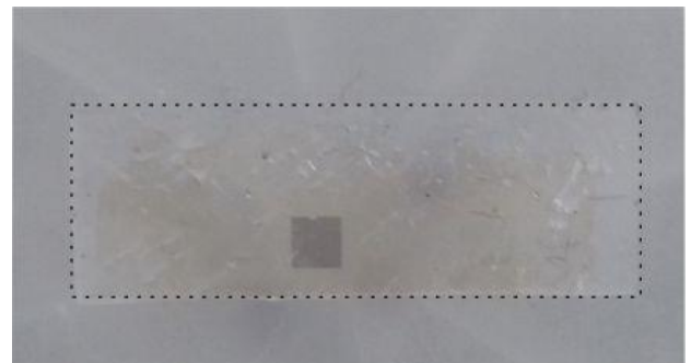
Fig. 1 Digital camera image of the Si nanoantenna (2 mm × 2 mm) embedded in a PDMS film. The dotted area denotes the PDMS edges.
