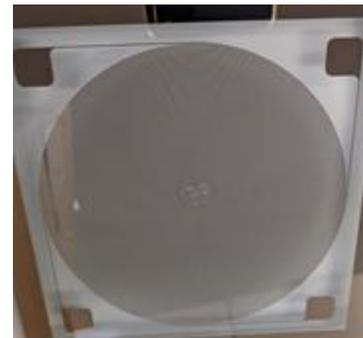
Fig. 2 Fabricated mask used for a following etching-process to create an electrostatic dust cleaning system.
