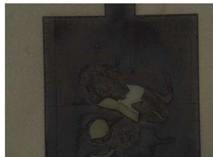
Fig. 1 Photo of substrate with 95nm BDD thin film after BDD film is peeled due to photo-resist peeling.
