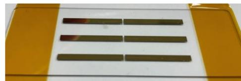
Fig. 1 Picture of the Au/Ti thin film electrode on the glass substrate.
