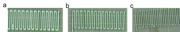
Figure 1 Trial pattern for the heater with the 500\ \text{nm} (a), 400\ \text{nm} (b), and 300\ \text{nm} (b) width.
