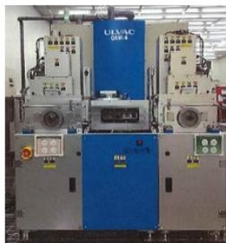
Fig. 1 Photograph of multi sputtering system
