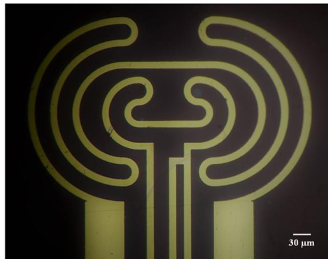
Fig. 1 Picture of electrode pattern fabricated on PI film
