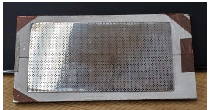
Fig. 2 Photograph of sensing element after Al sputtering with conductive film
