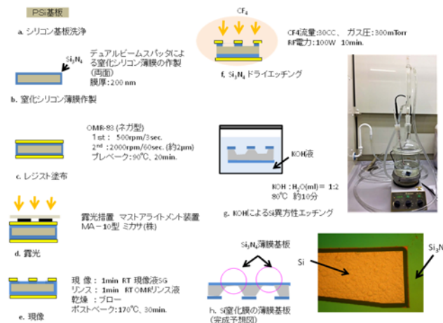
Fig. 1 Process flow chart of fabrication thin film substrate using Si anisotropic etching.
