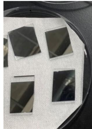
Fig. 1 Photograph of thin Al mirror on glass substrate
