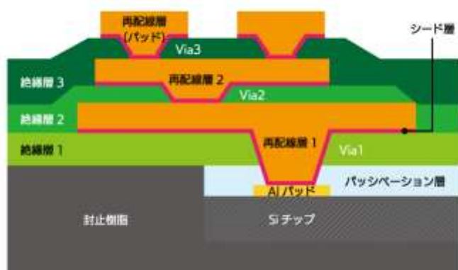
Fig.1 Fan-Out Wafer Level Package Cross-sectional structure
