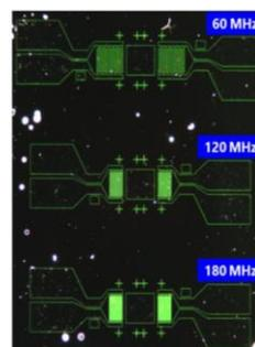
Figure 1. Picture of the sample after the electron-beam deposition.
