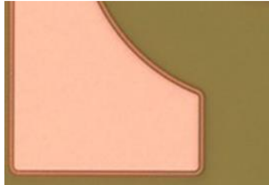
Fig. 1. Observation results of film peeling on ALD-Ta 2 O 5 on metal wiring.
