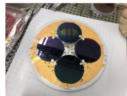
Fig. 1. Four samples set on jig.
