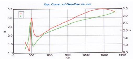
Fig. 3 Optical constant of TbCo/Pt thin layer (n : refractive Index, k : extinction coefficient)
