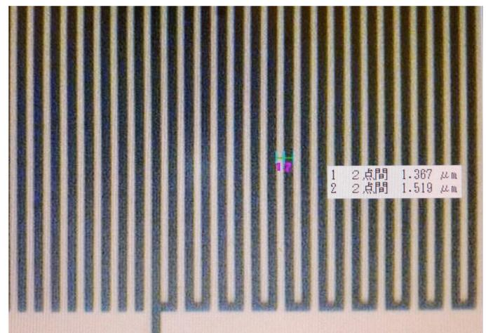
Fig. 1 Photo of IDT electrode (Design: Line=1.5 $\mu\text{m}$ , Space=1.5 $\mu\text{m}$ )
