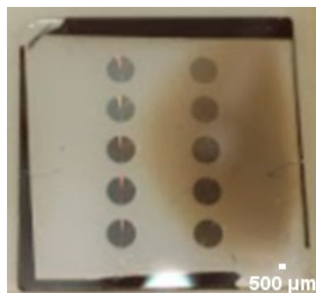
Fig. 1 Picture of the substrate after EB lithography and Si etching. The diameter of metalens is 2mm.
