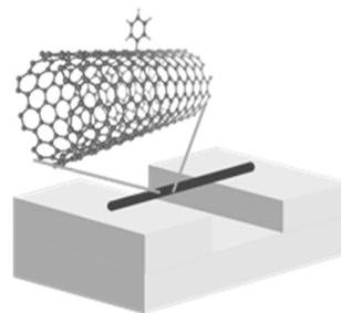
Fig. 1 Schematic of a functionalized Single-Walled Carbon Nanotubes (SWNT) suspended across a trench of SiO<sub>2</sub>/Si substrate.
