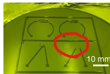
Fig.2 Picture of after endurance testing. The SU-8 mold is partially lost after PDMS pouring and releasing six times.
