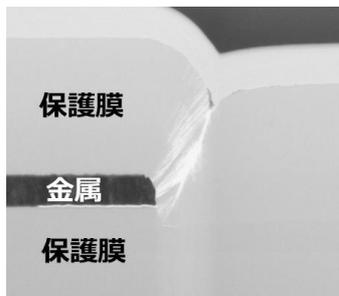
Fig. 1 TEM image of the edge of metal film.
