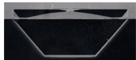
Fig. 2 Cross section view of micro heater.
