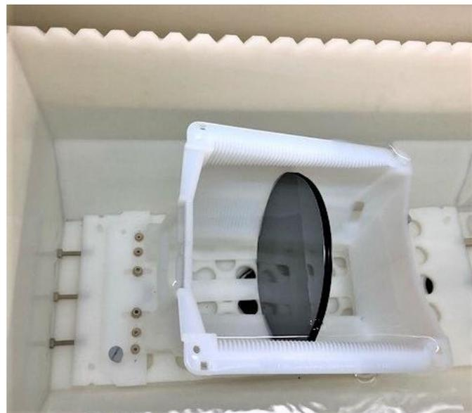
Fig. 1 Silicon wafers under cleaning.
