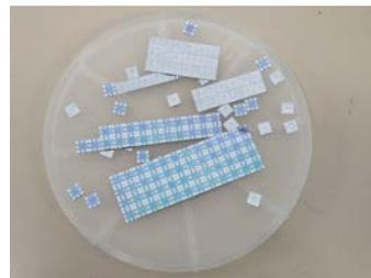
Fig. 1 Fabricated piezoresistive force sensor chips.
