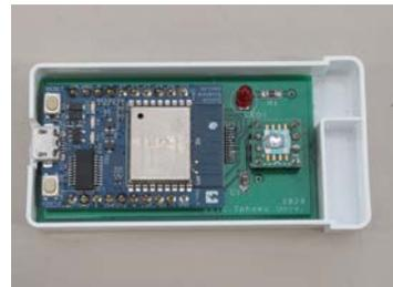
Fig. 2 IoT module including MEMS force sensor, Wi-Fi module, and peripheral circuit.
