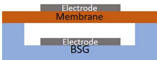
Fig. 1 Cross-section of Ultrasonic MEMS device.
