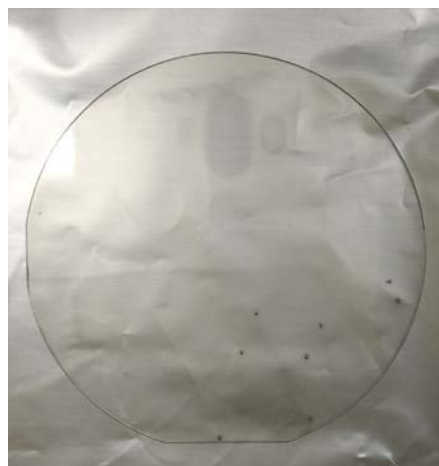
Fig.1 GaN wafer with SiO 2 film deposited by ALD
