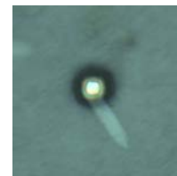
Fig.1 Optical microscope images of guanine crystal plate combined with ferromagnetic nanoparticles on Si/TbCo structure.
