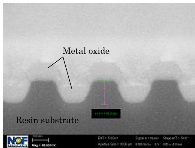
Fig. 1 Cross section of grating coupler in FIB-SEM
