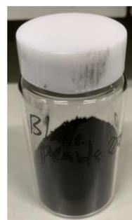
Fig. 1 Picture of the N-doped Nanocarbon Sample after Carbonization.
