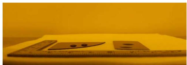
Fig. 2 Photography from the side of water droplets dropped on untreated  $\text{SiO}_2$  substrate and  $\text{SiO}_2$  substrate with plasma ashing treatment.
